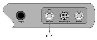
When an additional cable is inserted into output # 1 (electric output) the magnetic pickup signal is removed from the mix output so that there is now a separate output for both the magnetic and bridge transducer pickup systems.
