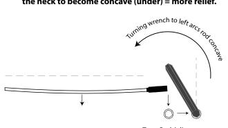
Truss Rod Adjustment
