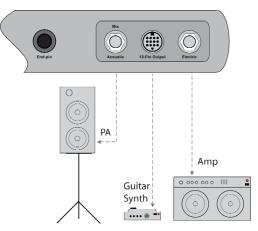
\*tip: when all three outputs are used you can insert a dummy plug into the "guitar out" jack on the guitar synth to remove the guitar from the synths's stereo output.
